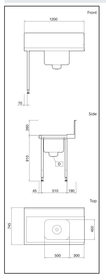
Handling System for Hood type Pre-wash Table with 500x400 Bowl and Strainer Left to Right, 1200mm
